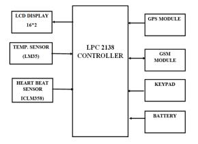
Fig.1. Block Diagram of Mobile Unit
