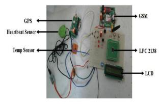
Fig.3. Hardware of mobile sensor unit
