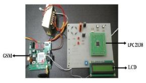
Fig.4. Hardware of server unit
